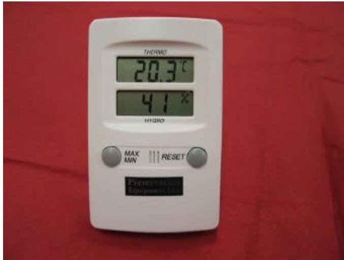
Device for monitoring temperature and humidity
